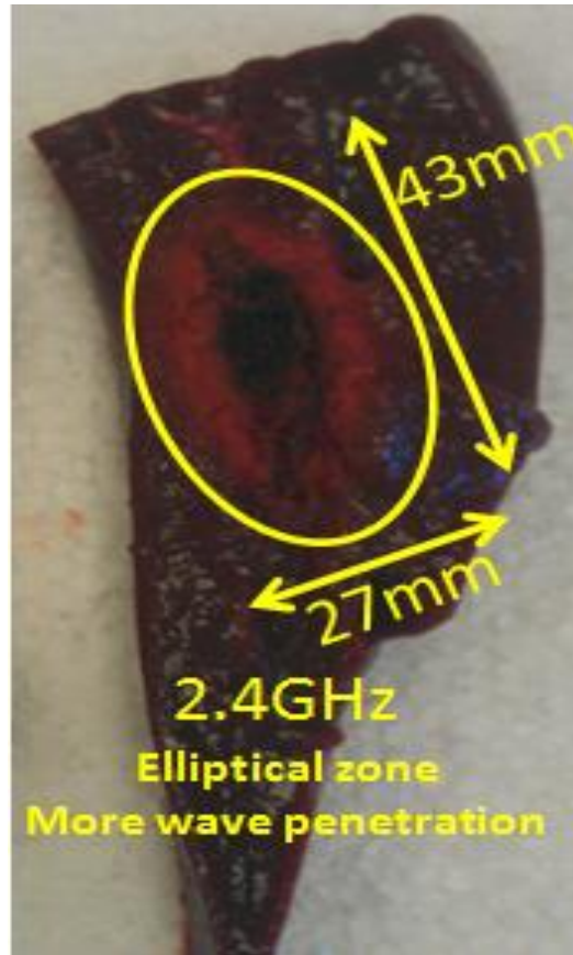
Figure 3.4 Ablation zone in ex-vivo pig liver at 2.4 GHz.
